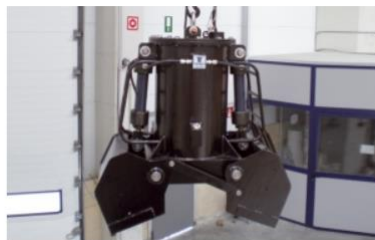
Electro-hydraulic clamshell grabs
